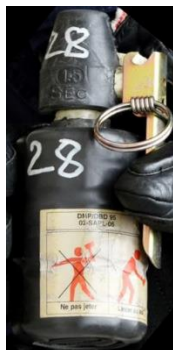
Figure 1: Undetonated DBD/95 with safety pin and fly off lever still intact
