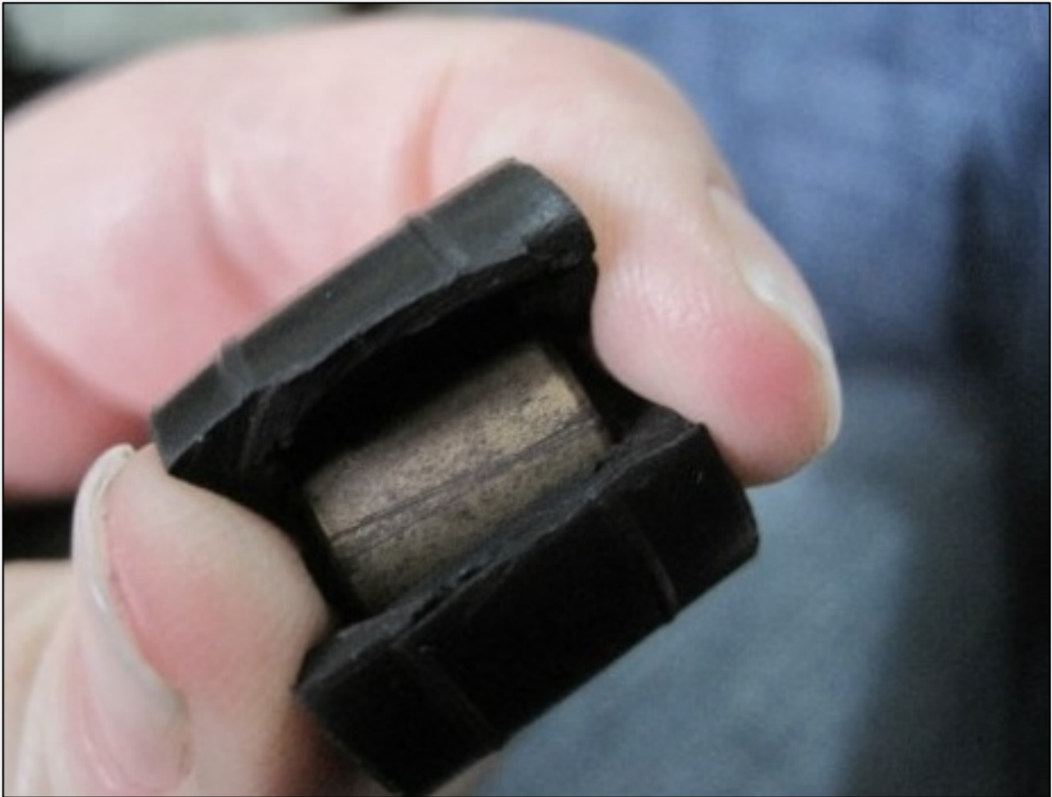
▲ Rubber coated metal bullet showing metal core
