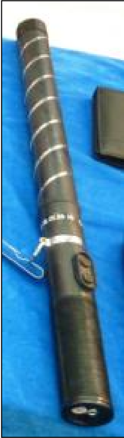
▲ Electric shock baton with metal spiral electrode
