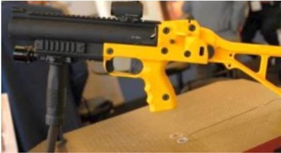
i) The Brugger and Thomet LL-06 (a less than lethal version of the GL-06): is a Swiss-made less than lethal grenade launcher that can be used with a range of different types of less-lethal ammunition, including CS gas, eXact iMPact rounds and dye marking canisters.
