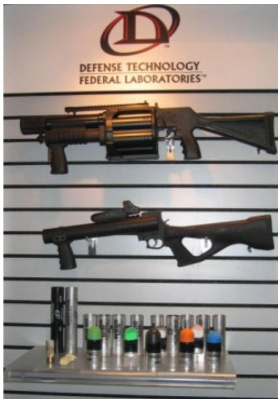
Defense Technology and NonLethal Technologies also manufacture a selection of launching devices including single-shot grenade launchers, multi-barrel / multiple shot grenade launchers, under-barrel grenade launcher attachments and launching "cups". The image on the left shows two types of Defense Technology launchers – a single shot launcher and a multi-barrel / multiple shot launcher photographed at Milipol 2005 – NonLethal Technologies also manufacture similar models.
