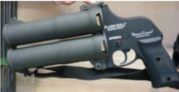
iii) The Flash-Ball SuperPro launcher: manufactured by French company Verney Carron, it can fire a wide range of 44mm ammunition, including rubber balls, soft rubber buckshots, dye balls and CS powder balls.
